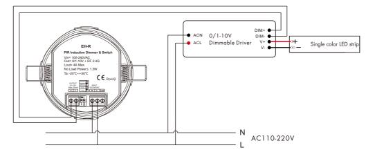
• Used as dimmer or switch, connect with 0/1-10V dimming driver (use AC OUT)
